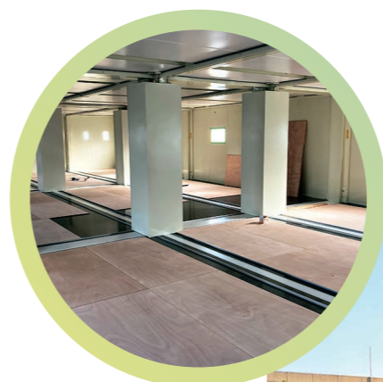
In hospitals lacking ICUs, medical containers are set up on the premises and used as hospital wards. The photos show a prefabricated ICU ward and its interior, which were preliminarily assembled in Japan. After this, it will be installed in a hospital in Kenya.
